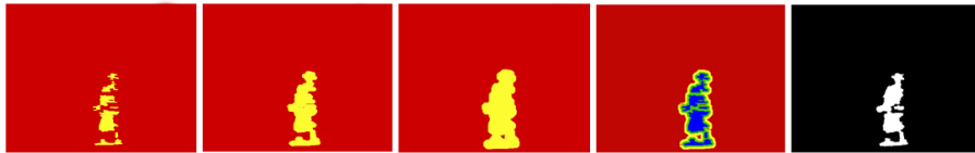
Figure 6: Illustration of the definition of the three pixels sets used by the GrowCut algorithm. The first column displays the initial foreground set (f), the second and third column show the masks m1 and m2, respectively. The fourth column presents the three associated sets: foreground set (f), unlabelled set (u) and background set (b) are coloured in blue, in green and yellow, respectively. The last column shows the final foreground after growth.
